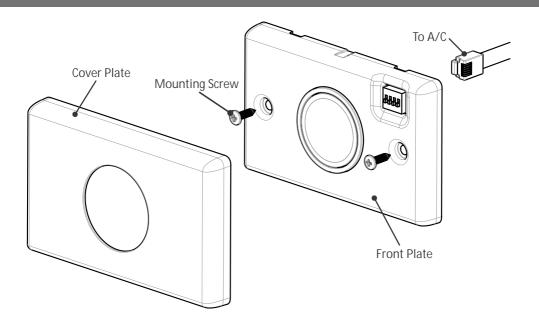
To remove Cover Plate once assembled onto the wall, use a small flat head screwdriver in the locations shown to pry Cover Plate off of the Front Plate.
