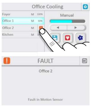
A fault for a Timer will be highlighted as shown.
