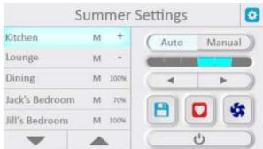
If a Motion Sensor and a Timer are both used for a Zone, the 'T' will override 'M'.
