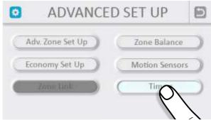
Zones with Motion Sensors and/or Timers are highlighted in green. If there is a fault with a Motion Sensor or Timer, it will be highlighted in red.
